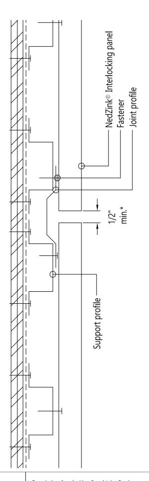
Check distance needed for expansion Interlocking panel.
